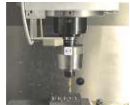
Mechatronic tool with integrated Minimal quantity lubrication
